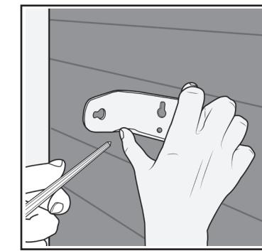
1. Determine the mounting location and line up the mounting bracket with the wall. Use a pencil to mark the pilot holes. Use a 1/16" drill bit to create the pilot holes (if mounting to drywall, use the plastic anchors included with the screws). Use a hammer to tap the plastic anchors into the pilot holes before screwing in the mounting bracket.
