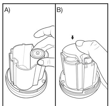
4. A) Insert 3 C-cell batteries and replace the door on the battery compartment. Ensure the batteries are inserted so that the flat ends are making contact with the springs.
