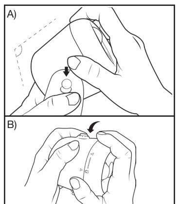
2. A) To release the bracket fully, keep the keyhole at a 45° angle and push the light down. The notch should slide down and release from the bracket.
