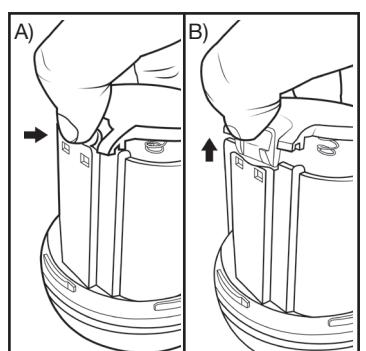
3. A) To release the door on the battery compartment, use your thumb to press the tab forward and lift.
