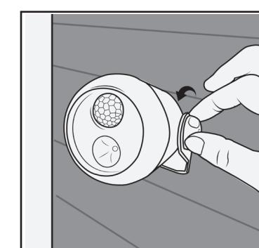
4. To change the direction of the light, loosen the thumbscrew and position the light in the desired direction.
