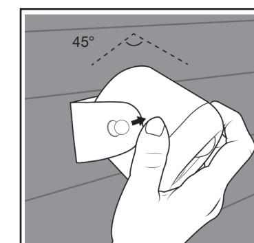
3. Place the notch on the side of the light through the large end of the keyhole and pull the light into place. On the other side of the light, replace the thumbscrew by rotating clockwise.
