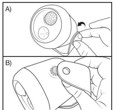
1. A) Remove the thumbscrew on the mounting bracket by twisting counterclockwise until it comes off.
